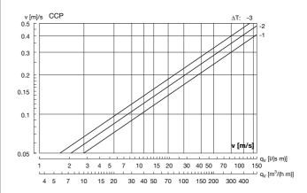
The speed is measured 0.5 m from the diffuser.
